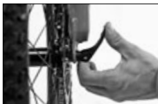
Image 6F(b) - Closing the Quick Release lever
