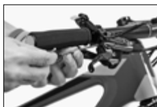
Image 4D(b) - Brake lever regulation
