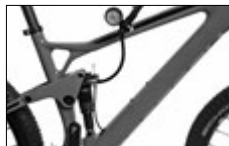
In the case of air suspension, it will be necessary to adjust the air pressure
