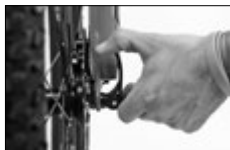
Image 6F(a) - Opening the Quick Release lever
