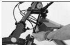
Setting the spring rate with a shock pump
