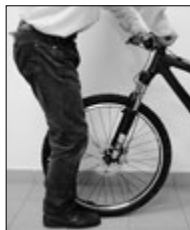
Image 3G - Testing of correct junction conditions stem-fork
