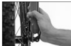
Image 6F(c) - Closing the Quick Release mechanism with the palm of your hand
