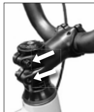
Image 3D - Minimum insertion mark of quill stem
