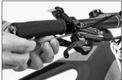
Adjusting the distance of the brake lever
