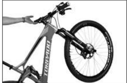
Lift the front wheel and make sure it swings easily
