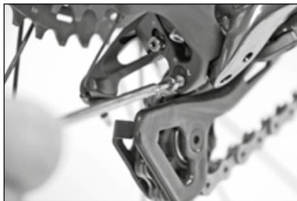
4. Turn clockwise to shift the pulleys inwards and anticlockwise if to shift them outwards.
