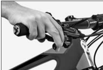
Gripping distance of the brake levers
