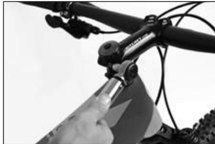
Retighten the clamping bolts on the sides of the stem with a torque wrench
