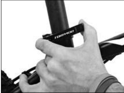
To set the seat height, it is necessary to loosen the seatpost clamping bolt or open the Quick Release
