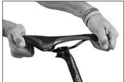
Check that the saddle which has just been tightened does not wobble
