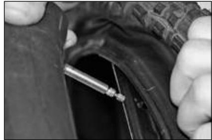
Insert the valve in the hole in the rim
