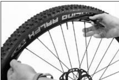
Slip the tyre lever in and lift the tyre bead by levering the rim
