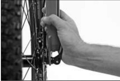
Closing the Quick Release mechanism with the palm of your hand
