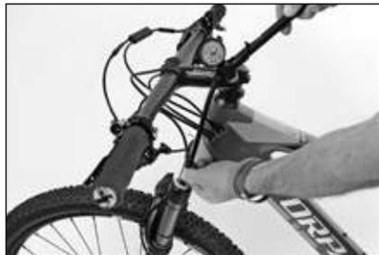
Setting the spring rate with a shock pump
