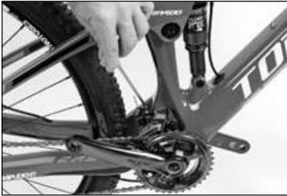
2. Use the limit screws to adjust the stroke of the derailleur.
