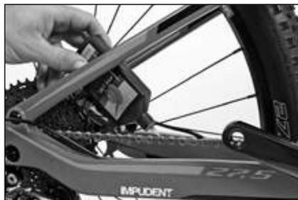
3. Turn the crank arm several times and allow a few drops to fall on the sprockets.
