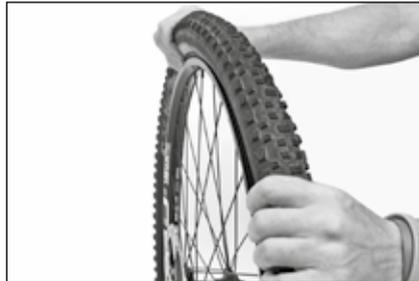
Press the tyre with both hands and check that the inner tube is not trapped under the tyre
