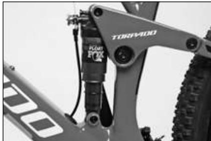
The displacement of the O-ring on the suspension shows the travel used
