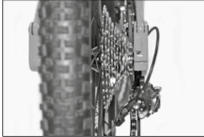
2. If it is not aligned, adjust the position with the limit screws. These are usually marked with an “H” (High) that indicates the biggest sprocket or with an “L” (Low) that indicates the smallest sprocket.
