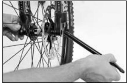
Removing through axles
