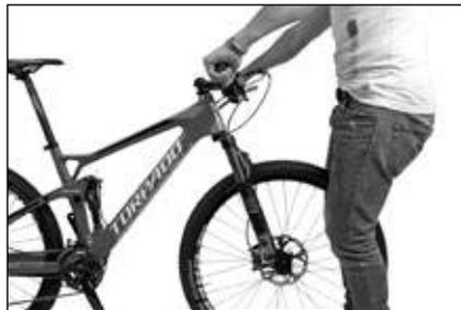
Try twisting the handlebars relative to the front wheel
