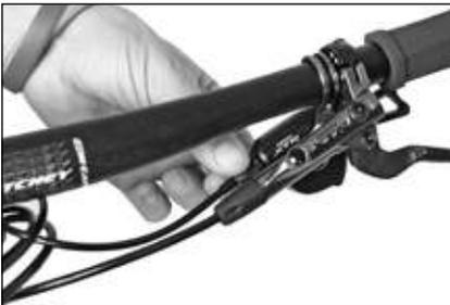
1. Adjust the tension using the screw through which the cable enters the shift lever.
