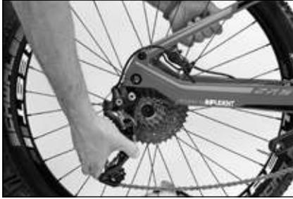
Check that the rear derailleur does not come into contact with the spokes
