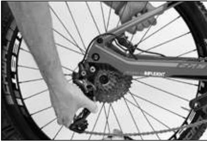
To remove the rear wheel, move the derailleur back slightly
