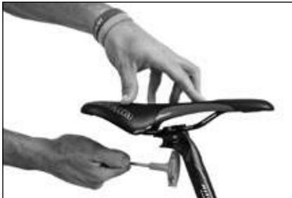
Loosen both bolts with two or three turns
