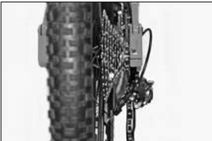
From behind, look at the cassette and check that the pulleys of the rear derailleur are perfectly aligned with the teeth of this sprocket
