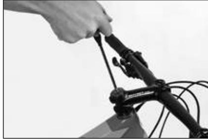
After loosening the clamping bolts on the sides, adjust the steering play with the countersunk adjusting bolt at the top
