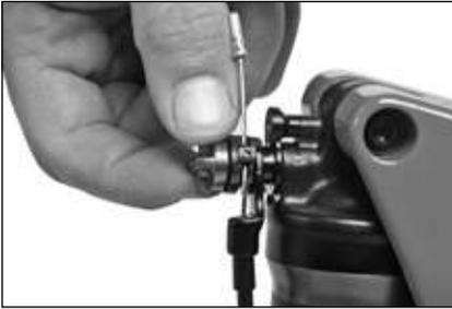
The damper is adjusted with an adjustment handwheel
