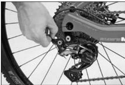
1. Adjust the tension of the cable by turning the adjustment bolt.
