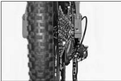
Move the chain onto the smallest sprocket
