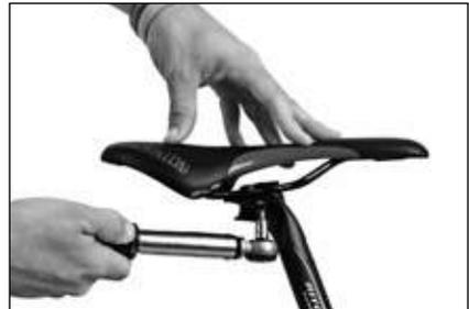
Tighten both bolts gradually and alternately without exceeding the maximum torque allowed
