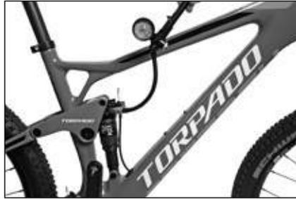
In the case of air suspension, it will be necessary to adjust the air pressure
