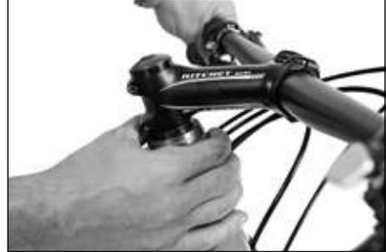
To check the play for the headset, pull the front brake, push the Torpado MTB back and forth while placing your hand on the head cup
