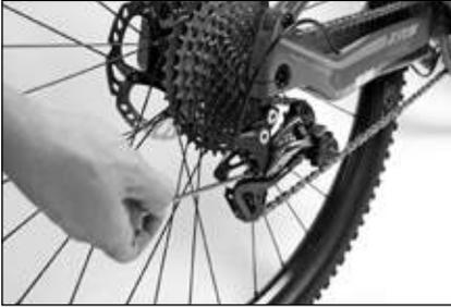
7. Check the position of the rocker arm compared to the cassette. There should be enough clearance room for at least one or two links between the pulley and the largest sprocket. If not, adjust this gap by turning the screws on the rear derailleur, located on the front side of the drop-out.
